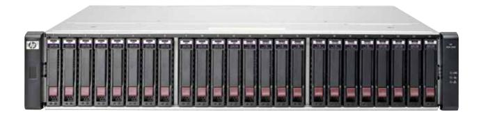
High-performance 8/16 Gb Fibre Channel (FC) array delivering entry-level and mid-market features to traditional MSA customers through Solid State Drives (SSDs) and latest host interconnects. Simple to deploy and simple to manage.
